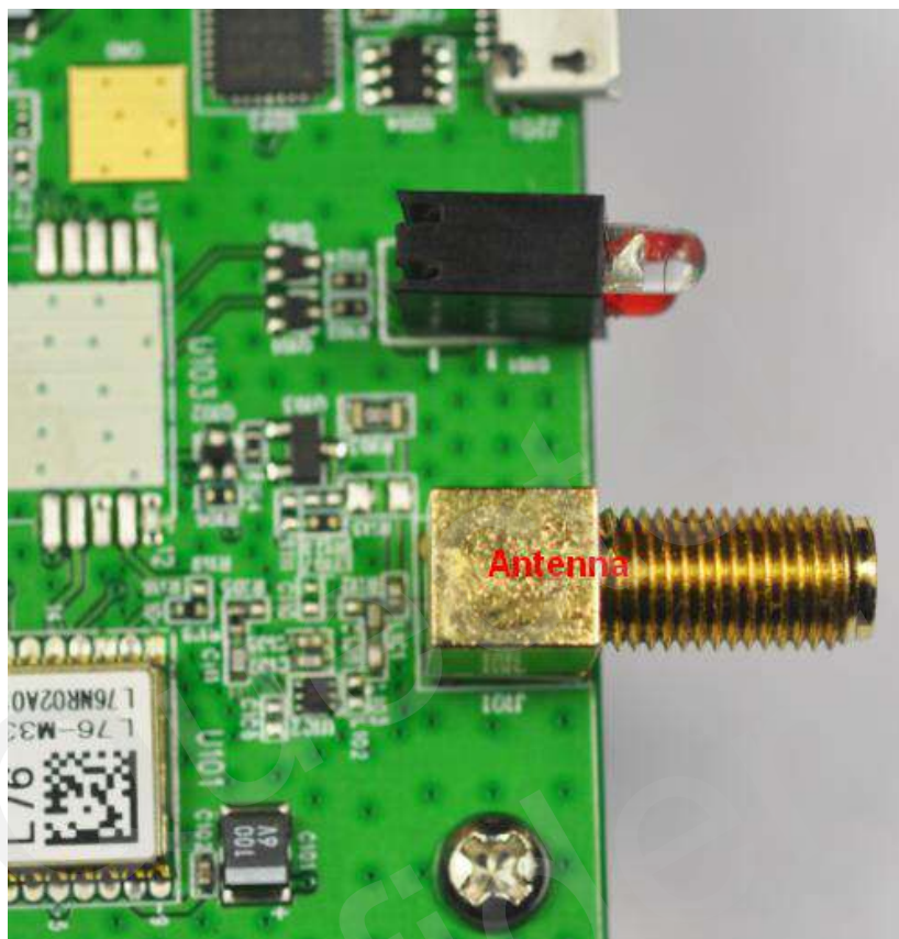
Figure 6: L76 EVB Antenna Interface
